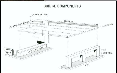
38. **Bridge Rail** - A bridge parapet or a barrier attached to a bridge deck to restrain motor vehicles, pedestrians, or other users. This includes guardrails which serve as bridge rails.
